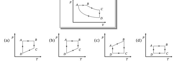
Solution : (a) AB is isobaric process, BC is isothermal process, CD is isometric process and DA is isothermal process
